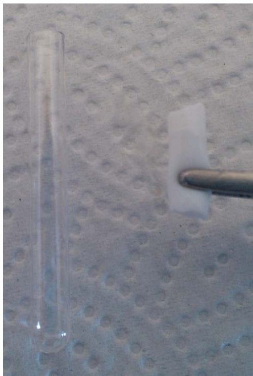
Fig. S5. Image of centrifuge tube (Ultra-Clear™ 5*41 mm ) and polyacrylamide hydrogel prepared inside the centrifuge tube.
