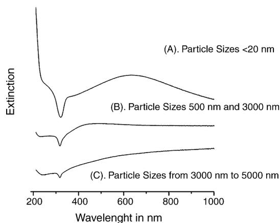
Fig. 4. UV/VIS measurements of silver particles: (a) silver particles with sizes, <20 nm, synthesised with iron ammonium citrate as reductant; (b) silver particles with 500 and 3000 nm in diameter, synthesised with ascorbic acid as reductant and PVP K 25 as stabilising agent; and (c) silver particles with sizes in the range from 3000 to 5000 nm in diameter, synthesised with ascorbic acid as reductant and Tamol VS as stabilising agent.
