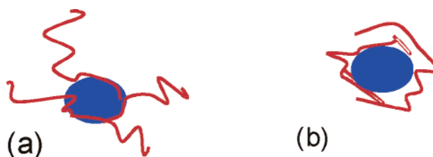
Figure 3. Stabilization of primary particles by (a) Lutensol and (b) Pluronic.
